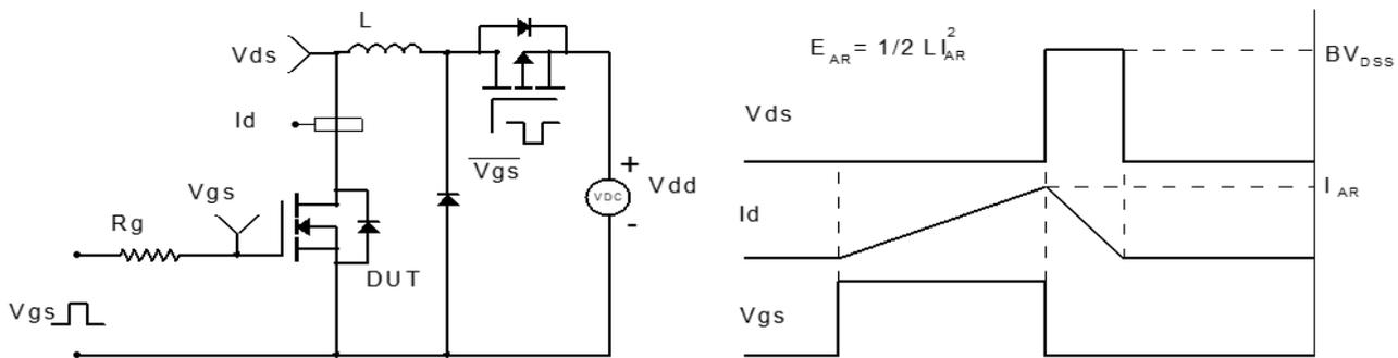
Figure 3: Unclamped Inductive Switching Test Circuit & Waveform
