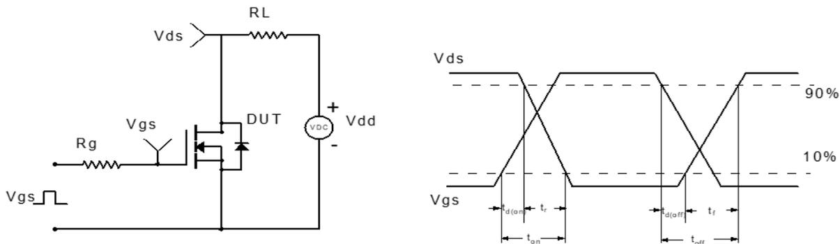
Figure 2: Resistive Switching Test Circuit & Waveform
